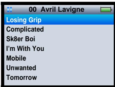
Song positions within the playlists are the same for track selections. The very first song at the top is track 01, the next song is track 02 and so on. You can have up to 99 songs in each playlist. The iPod is capable of playing most standard audio formats such as AAC, MP3, MP3 VBR, Lossless, WAV and AIFF.
