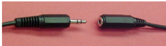
Audio Connector 3.5mm Stereo (1/8"), Tip is right-channel audio
