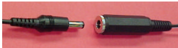
DC Power Connector Barrel type 2.1mm x 5.5mm, Center pin positive
