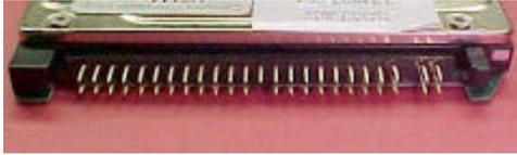
The hard disk drive has two sets of connector pins. 43-pins on the left side and 4-pins on the right.
