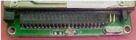
Slide the disk drive forward into the connector. The 4-pins on the right are not used.
