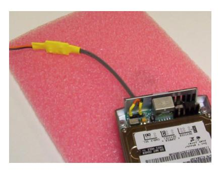
The CD100 external mute accessory has a short (3") set of wires on one end and a long 36" set of wires at the other.
