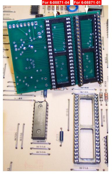
At the bottom side of the tester board are two 40-pin IC sockets. Two 20-pin strip headers will be inserted into one of these sockets. The board under test here is part # 6-08871-01 which uses the U2 socket position. Gently press the pin strip into the socket, being careful not to bend the pins.
