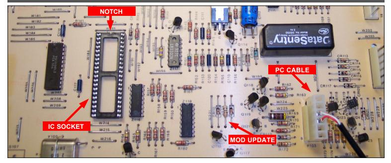
To use the Troubleshooter, you need to remove the custom microprocessor chip and insert a 40-pin IC socket. A low profile, dual leaf type socket, such as 3M part number 4840-6004-CP, is recommended.
