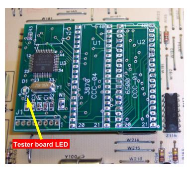
Now insert the tester board into the IC socket. Make sure the pins line up with the socket then gently press down.
