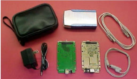
Your kit comes with a USB external HDD circuit board, MP3-DSP digital music player circuit board, PC connector cables, jukebox connector cables, enclosure, power supply and a storage pouch.
