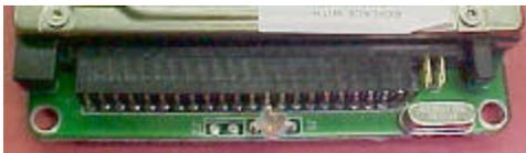
Slide the disk drive forward into the connector. The 4-pins on the right are not used.
