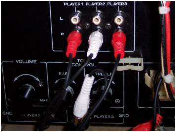
2) Take 2nd Y-cable, connect one male plug to Player 3, the other to female end of 1st Y-cable. Connect the red male plug from player to the female end of 2nd Y-cable.
